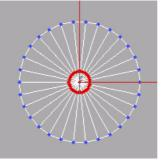
5. In the front view, select the vertices on the perimeter of the cylinder that are just above the vertices in the midsection of the circle.
