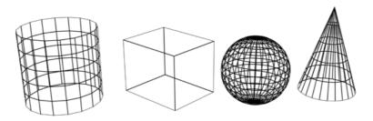
Geometric Primitives: cylinder, cube, sphere and cone
