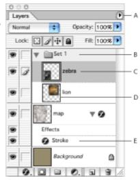
Photoshop Layers palette: A. Layers palette menu B. Layer set C. Layer D. Layer thumbnail E. Layer effect
