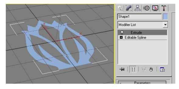
• To make it become a 3D object, we amend the parameter of the Extrude modifier to add depth to the shape.
